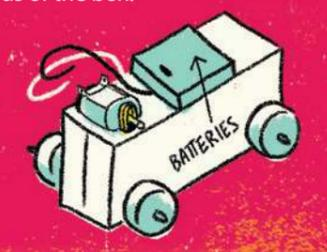
**8** Check the battery holder is switched off, then attach the wires to the motor terminals. Hook the wire round the terminal and make sure the shiny metal of the wire is in contact with the shiny metal terminal. Use a piece of sticky tape to secure it.
