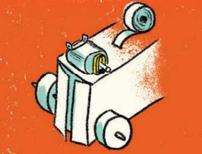
**7** Finally, stick the battery holder on top of the box, put it towards the middle but so the wires can still reach the terminals on the motor. Make sure you can access the switch! Close the ends of the box.
