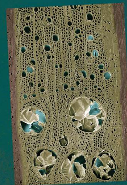
Cross-section of heartwood (central supporting pillar) of the oak Quercus robur , using an electron micrograph. The largest vessel is actually 0.3 mm in diameter.
